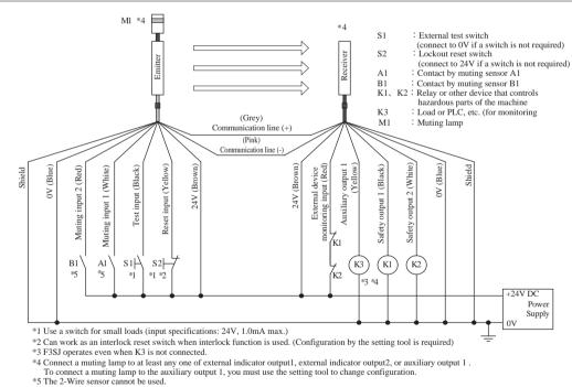
■ Wiring when external device monitoring function is not required
