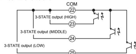
KM50-E's 3-STATE function can sort the integration condition of electric energy into HIGH, MIDDLE and LOW by setting HIGH threshold (4 I.H.L.H) and LOW threshold (4 L.L.H). This function allows you to grasp power consumption state and supports extracting power loss.
