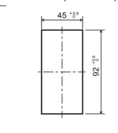
Mount the Product such that the display can be seen properly from the front. To fix the Product to the panel, use the attached mounting bracket.
