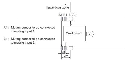
A workpiece finished passing the muting sensor A1 and the sensor starts turning OFF. For standard muting system, muting is released here. For exit only muting, F3SJ's safety function is disabled for a exit only muting delay time: T5.
