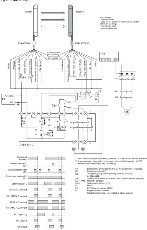
\* Output operation mode of auxiliary output 1 is "safety output information/reverse enabled" (initial setting)
