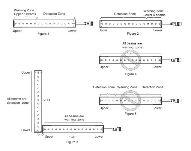
Setting Example: Configuring a warning zone information for auxiliary output 1 Reverse Output: None
