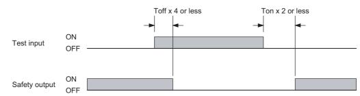
Ton: Response time of safety output's OFF to ON, Toff: Response time of safety output's ON to OFF
