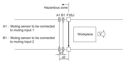
A workpiece passed F3SJ's detection zone. When muting end waiting time: T4 (0.1s) passed after F3SJ received light, muting state is released.
