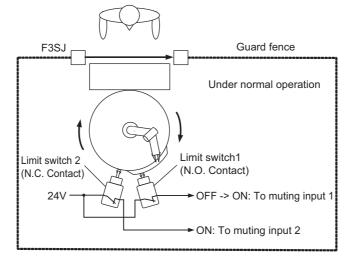
Rotation of a robot arm sets the muting input 1 from OFF to ON. Safety function of F3SJ is enabled.
