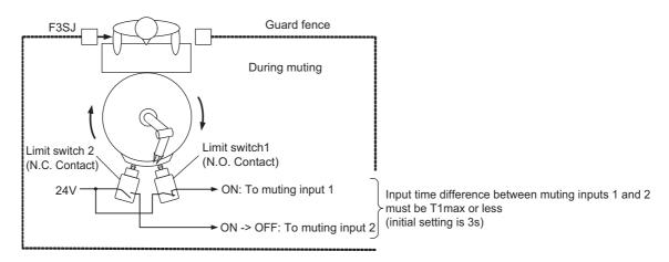
When the muting input 1 turns from OFF to ON and when the muting input 2 is turned from ON to OFF within T1max [s] before or after the muting input 1's turning ON, safety function of F3SJ is disabled. (Safety output is kept ON even if F3SJ is blocked)
