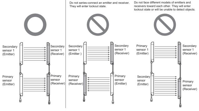
Connect an emitter to another emitter, and a receiver to another receiver, as shown below.
