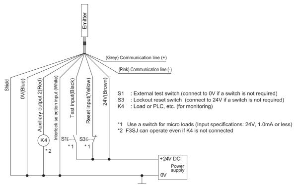
Wiring When External Device Monitoring Function Is Not Used 1.Disabling external device monitoring function by the setting tool
