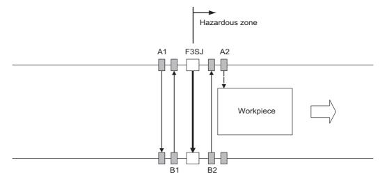
Muting sensor A2 is turned OFF and the muting function is released, and the safety function of the F3SJ is working.
