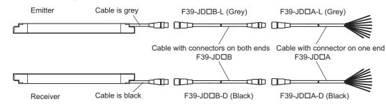
■ Cable with Connectors on Both Ends: Cable for Connection with G9SA-300-SC (F39-JC□C, sold separately)
