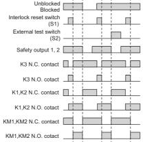
Note 1) F3SJ's external device monitoring and auxiliary output cannot be used. Note 2) S2 performs normal operation when opened and external test when short-circuited. Note 3) Do not connect any cable to terminals C1, D1, D2, E1, and E2
