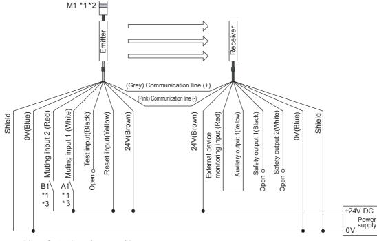
Contact by muting sensor A1 A1 B1 Contact by muting sensor B1
