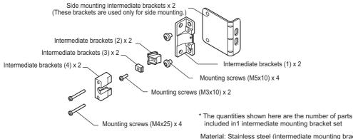
Material: Stainless steel (intermediate mounting bracket) Zinc die-cast (Intermediate mounting brackets (1) to (4)) Iron (mounting screws)
