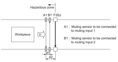
All muting sensors are turned OFF and the safety function of the F3SJ is working.
