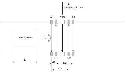
d2: Maximum distance required for the muting sensor to keep the muting function enabled D2, D3: Minimum distances required for the muting sensor to keep the muting function enabled
