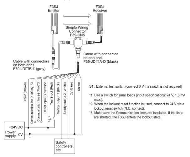
Note1: When using the Simple Wiring Connector (F39-CN5), the following functions are not available. • Manual Reset
