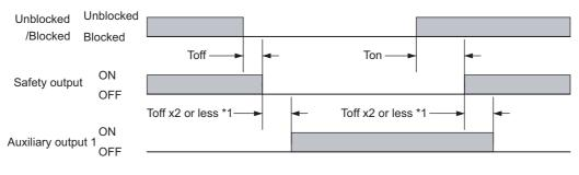
\*1 When a reversed signal of safety output is assigned to the auxiliary output 2 by the setting tool, a delay time of the auxiliary output 2 from the safety output is Toff x 3 or less.
