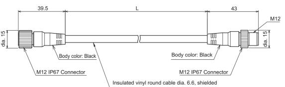
8-wire (4-pair) (Cross section of conductor: 0.3mm<sup>2</sup>/ Insulator diameter: 1.15mm)
