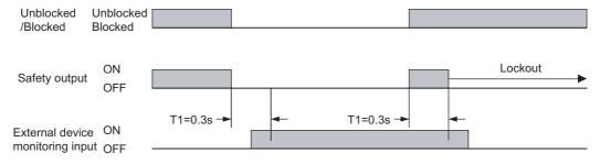
T1: Allowable delay time (can be changed by the setting tool. 0.1 to 2.5s)
