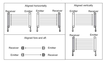
If 2 sets are installed near each other, reflection from the surfaces may cause mutual interference. For such a case, it can be improved by reducing operating range through the setting tool (see Step 3).
