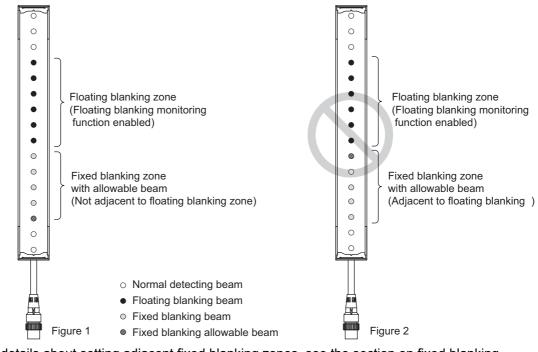
\*2 For details about setting adjacent fixed blanking zones, see the section on fixed blanking.
