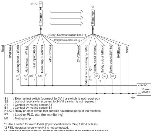
\*3 Connect a muting lamp to external indicator output of an emitter or a receiver.
