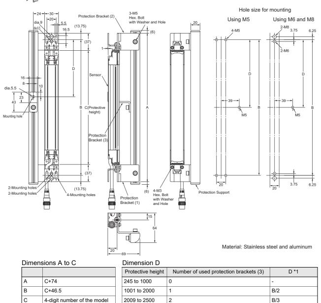
\*1 D is for reference and must be a length that should not affect intermediate mounting bracket
