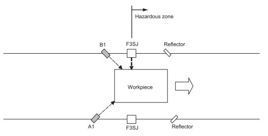
The F3SJ is blocked but the safety function is disabled by the muting function, and safety outputs 1 and 2 are turned ON.
