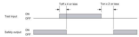
Ton: Response time of safety output's OFF to ON, Toff: Response time of safety output's ON to OFF 1/2 Response time p.12
