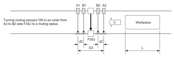
This arrangement example uses regressive reflection type E3Z-R□□ series as a muting sensor. Arrangement must take mutual interference into account.
