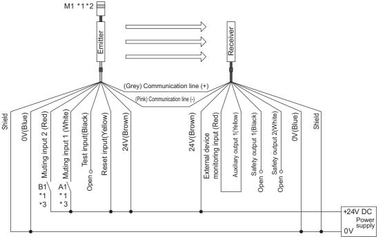
A1 B1 : Contact by muting sensor A1 : Contact by muting sensor B1
