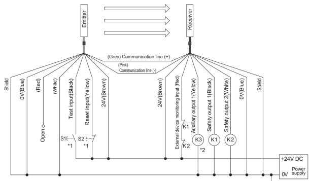
S1 : External test switch (connect to 0V if a switch is not required)
