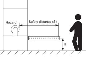
Also, you must include a hazardous condition under which a person may go through under a detection zone carelessly if it exceeds 300mm (200mm for other purpose than industrial use) into risk assessment.
