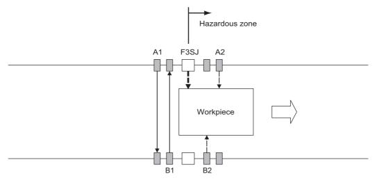
Muting sensors A1 and B1 are turned OFF but A2 and B2 are ON, so the muting function is still working. Safety outputs 1 and 2 are turned ON.
