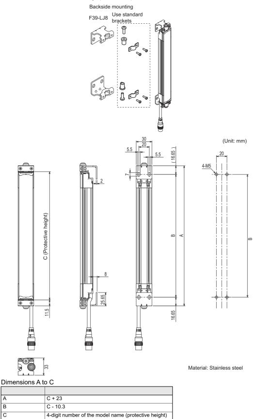
The F39-LJ8 and intermediate mounting brackets cannot be mounted simultaneously, so set the protective height to
