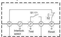
Wiring when not using external device monitoring function
