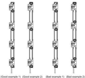
Mount One-touch M6 Brackets (or One-touch M8 Brackets) according to the mounting positions of the emitter and receiver. The positions of Intermediate Brackets mounted to the emitter and receiver must be aligned with each other.
