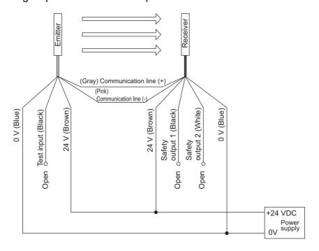
■ Wiring when using test input line
