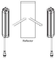
Position with detection zone bent at 90°
