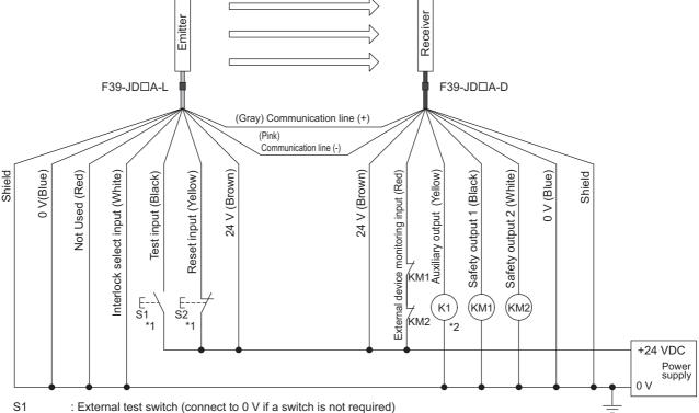
: Lockout reset switch (connect to 24 V if a switch is not required) KM1, KM2: Safety relay with force-guided contact (G7SA) or magnetic contactor
