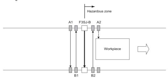
Muting sensor B2 is turned OFF, the muting function is released, and the safety function of the F3SJ-B is enabled.
