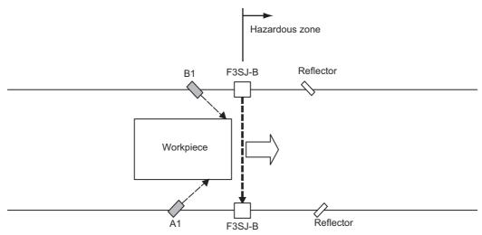
When muting sensors A1 and B1 are turned ON in this order, the muting function is enabled. In this state, the safety function of F3SJ-B is disabled.
