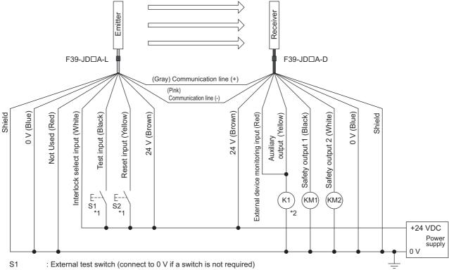
S2 : Interlock/lockout reset switch
