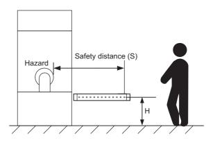
Also, you must include a hazardous condition under which a person may go carelessly through under a detection zone if it exceeds 300 mm (200 mm for other purpose than industrial use) into risk assessment.
