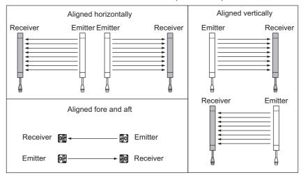
If two sets of F3SJ-E/Bs are installed near each other, reflection from the surfaces may cause mutual
