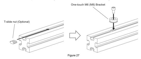
**4.** The positions of Intermediate Brackets mounted to the emitter and receiver must be aligned with each other.
