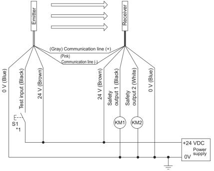
: External test/lockout reset switch (connect to 0 V if a switch is not required) KM1, KM2 : Safety relay with force-guided contact (G7SA) or magnetic contactor
