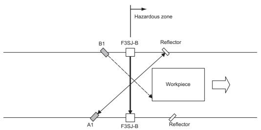
Muting sensor A1 is turned OFF, the muting function is released, and the safety function of the F3SJ-B is enabled.
