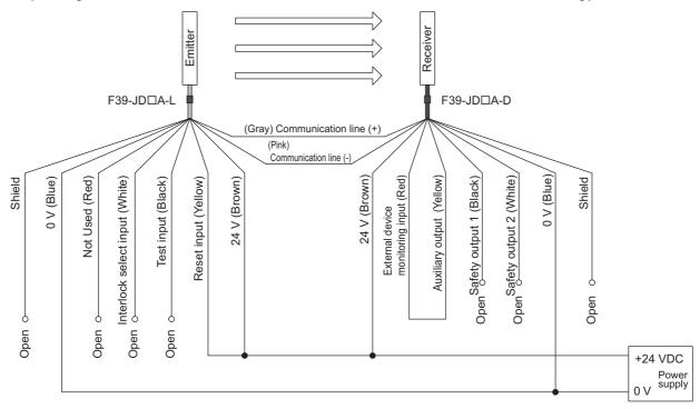
■ Wiring when using manual reset mode and external device monitoring
