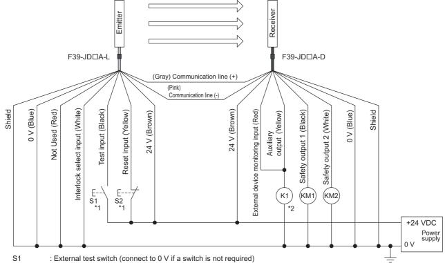
S2 : Lockout reset switch (connect to 24 V if a switch is not required) KM1, KM2: Safety relay with force-guided contact (G7SA) or magnetic contactor
