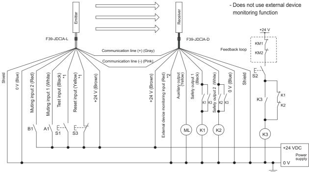
S1 : External test switch (connect to 0 V if a switch is not required)
