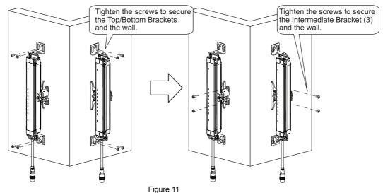
Screws to mount the brackets to the wall are not included.
