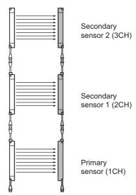
Properly connect an emitter to another emitter, and a receiver to another receiver, as shown below.
