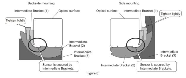
**3.** Attach a Top/Bottom Bracket and lightly tighten it using the included hexagon socket head cap screws (M3x6).
