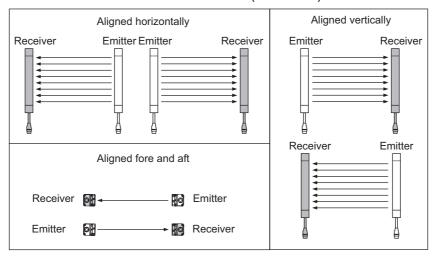
If two sets of F3SJ-Bs are installed near each other, reflection from the surfaces may cause mutual
