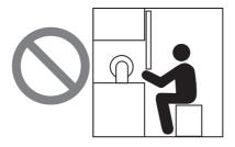
A person is between the sensor's detection zone and the hazardous zone of a machine.
