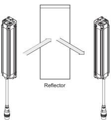
Position with detection zone bent at 90°
