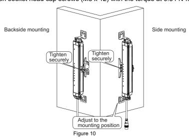
**5.** Tighten the screws to mount to the wall by the order of Top/Bottom and Intermediate Brackets. (Figure 11)
