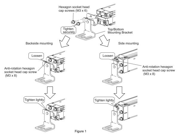
**2.** Adjust the Top/Bottom Brackets to the mounting position of the wall surface and then tighten them with screws. (Figure 2)
