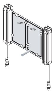
□When muting function is used, installation condition of muting sensor must not be changed.
