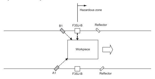
The F3SJ-B is blocked but the safety function is disabled by the muting function, and safety outputs 1 and 2 are turned ON.
