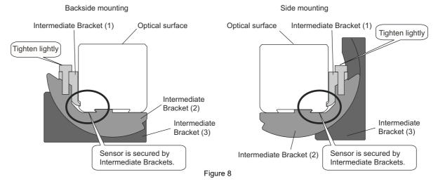
3. Attach a Top/Bottom Bracket and lightly tighten it using the included hexagon socket head cap screws
