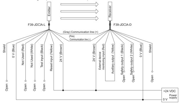
■ Wiring when using external device monitoring
