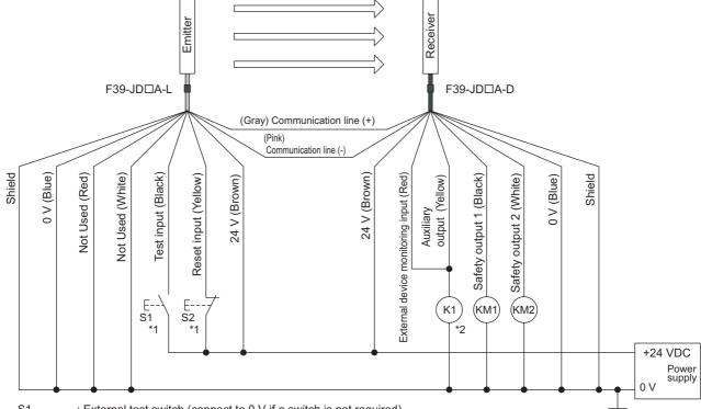
S1 : External test switch (connect to 0 V if a switch is not required) S2 : Lockout reset switch (connect to 24 V if a switch is not required) KM1, KM2: Safety relay with force-guided contact (G7SA) or magnetic contactor
