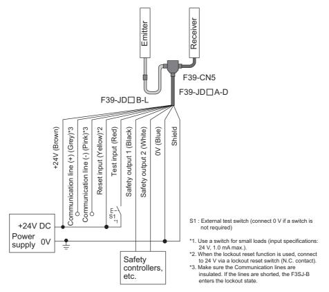
Note1:When using the Simple Wiring Connector (F39-CN5), the following functions are not available.
