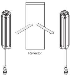
Position with detection zone bent at 90°
