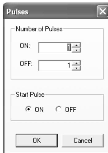
3. Set the number of pulses and the start pulse, and then click the **OK** Button. The specified pulses will be applied to the selected area.
