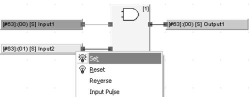
As shown below, input 1 and input 2 turn ON and the AND function block output (output 1) turns ON.
