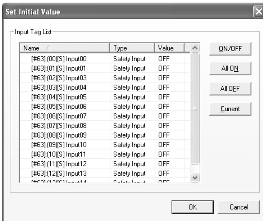
2. Select an input tag to set the initial value for debugging. To select more than one tag, hold down the **Shift** Key or the **Ctrl** Key while selecting tags with the mouse.
