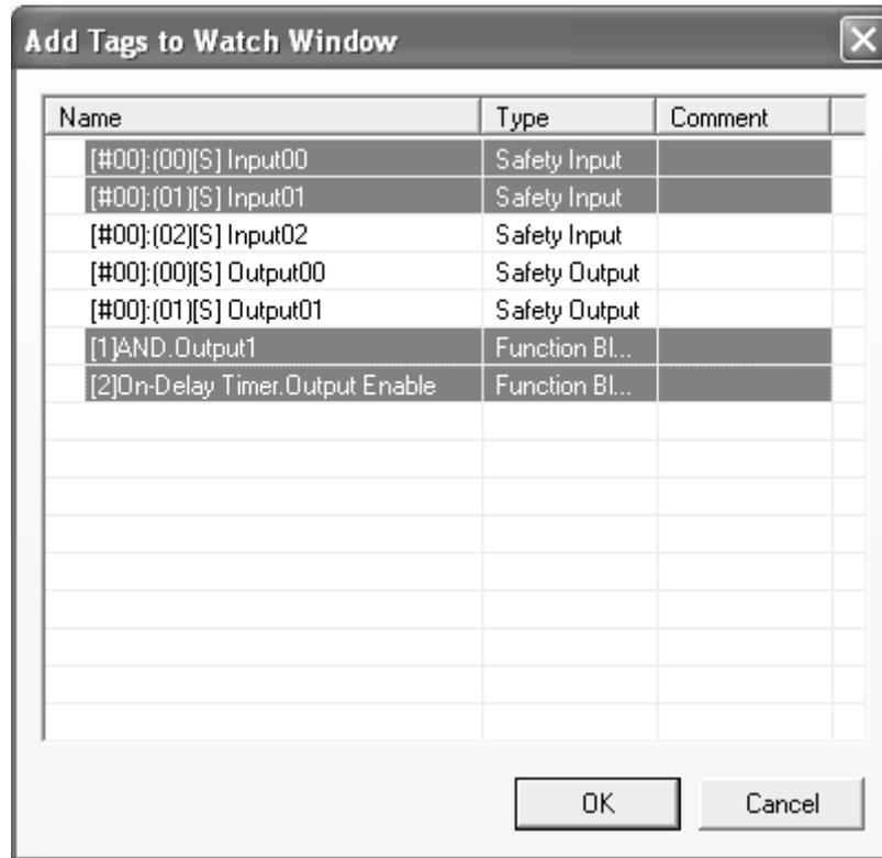
3. Select the tag to be added to the Watch Window and click the **OK** Button. More than one tag can be added at the same time by holding down the **Ctrl** Key or **Shift** Key while selecting the tags.
