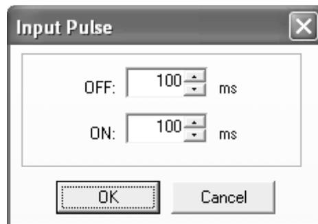
3. Enter the OFF and ON times and click the **OK** Button. The time settings for both the OFF and ON times must be between 100 and 10,000 ms. The time setting specified here is the program time. Simulation with the Logic Simulator will be executed based on the time set here, multiplied by the cycle time base value.
