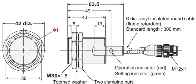
\*1. The E2EF-QX□D type Clamping nut (optional accessory) is grooved to identify the material (SUS303, with fluororesin coating).
