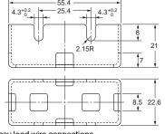
Note: The Cover has six holes for easy lead wire connections.
