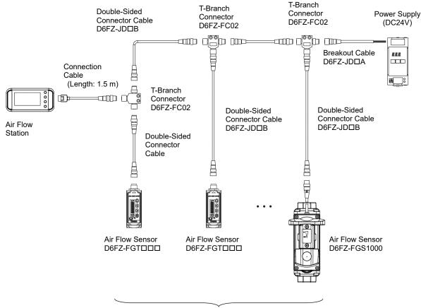
Max. 8 Air Flow Units can be Connected
