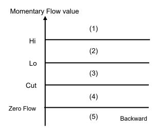
The Air Flow Sensor thresholds are set to the following values by factory default:
