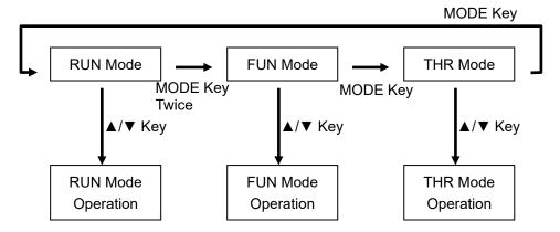
The Air Flow Station provides the three operation modes, which can be switched with the MODE key.
