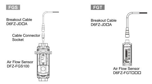
[2] Connect the following breakout cable wires to the upstream unit as required.
