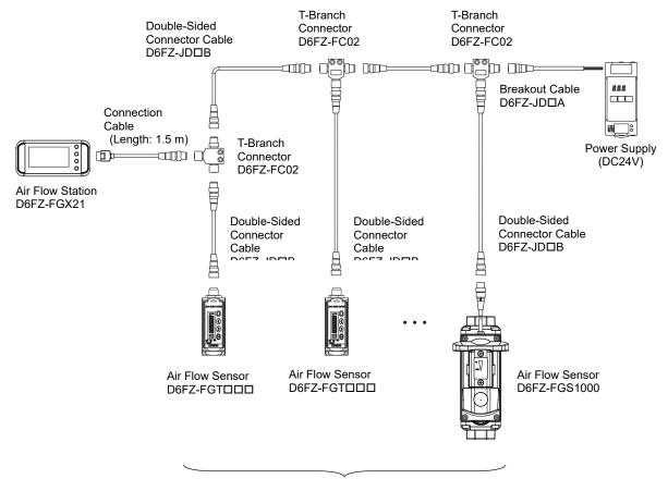
Max. 8 Air Flow Units can be Connected
