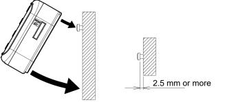
Enlarged Hook Screw Section View
