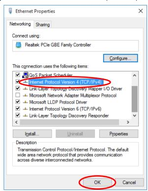
[6] Select "Use the following IP address" and set "IP address" and "Subnet mask". Click "OK" to close the window.
