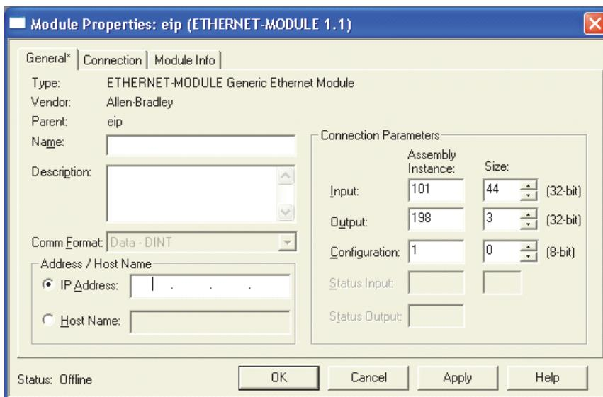
6. Configure the “Required Packet Interval (RPI)” and click OK. 20 ms or slower is strongly recommended. 10 ms is the minimum allowed by QX-870:
