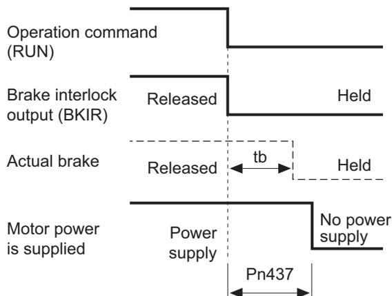
Make the setting as follows to prevent the machine (workpiece) from moving or falling due to the delay time in the brake operation (tb).
