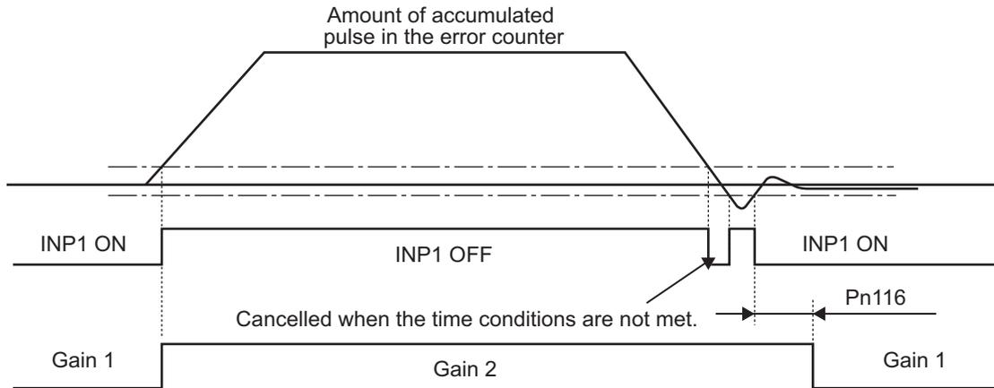
● **Gain Switching Mode = 10: Switching by Combination of Position Command Input and Speed**
