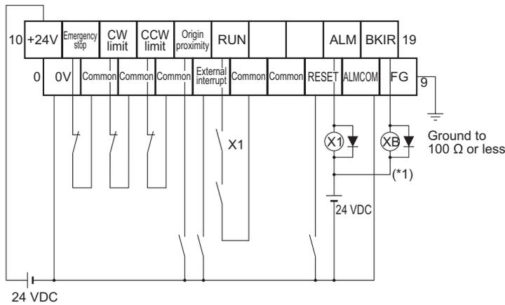
\*1 The XB contact is used to turn ON/OFF the electromagnetic brake.
