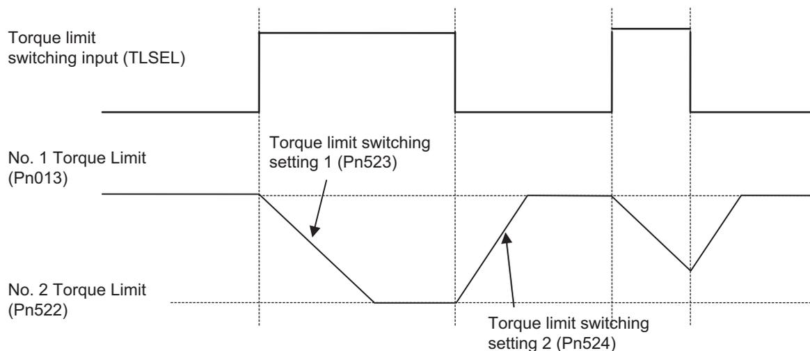
If the No. 1 Torque Limit (Pn013) or No. 2 Torque Limit (Pn522) value is changed from the front panel or CX-Drive, the rate of change setting is ignored and the new torque limit value is applied immediately.
