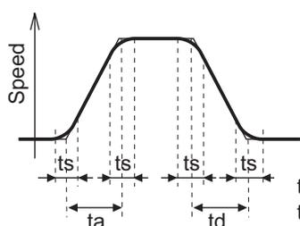
1. Set the acceleration time and the deceleration time for the basic straight-line portion in Pn312 and Pn313.
