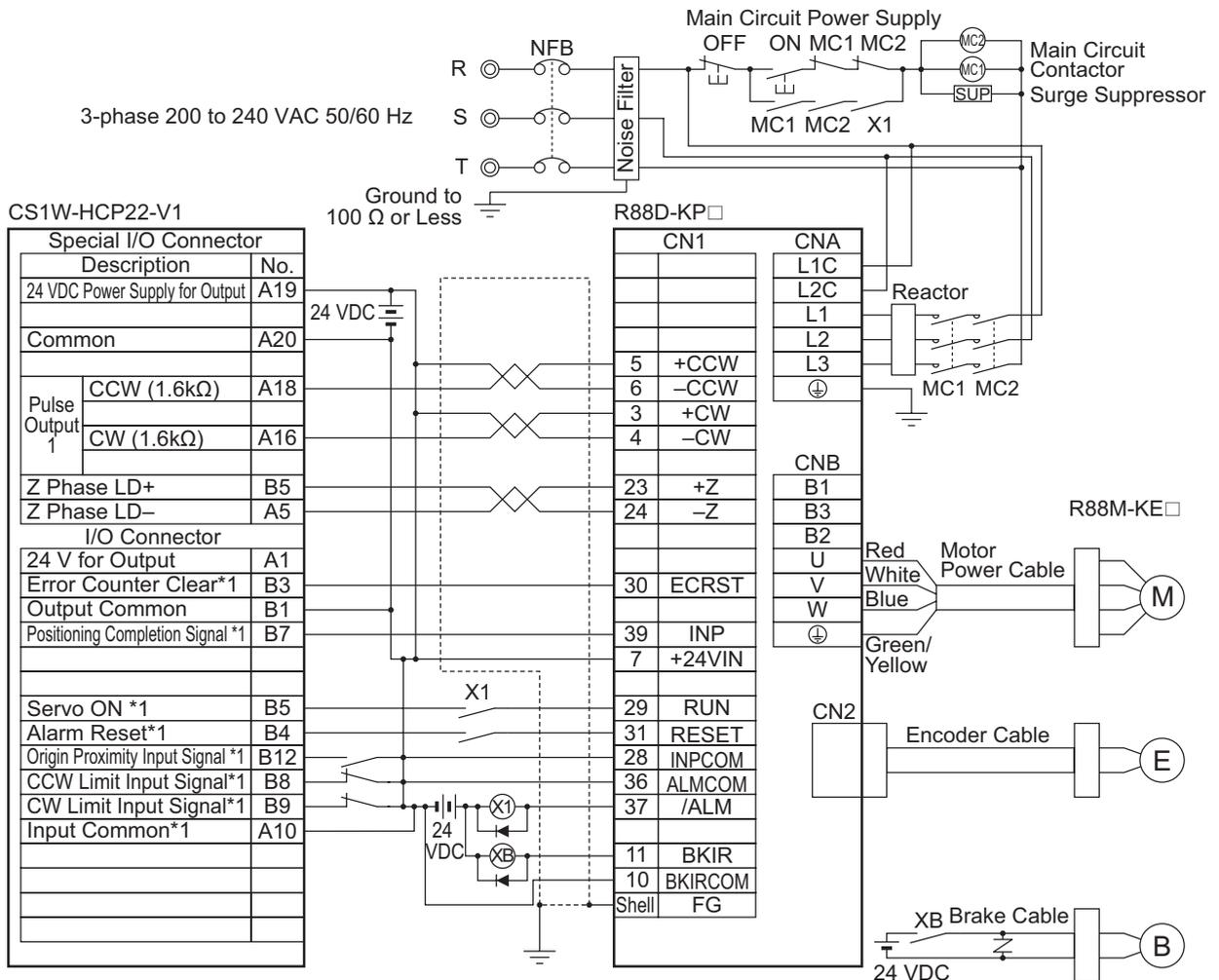
\*1 The I/O signals for the HCP22 vary depending on the allocations of internal relay areas. Change the wiring according to the allocations.
