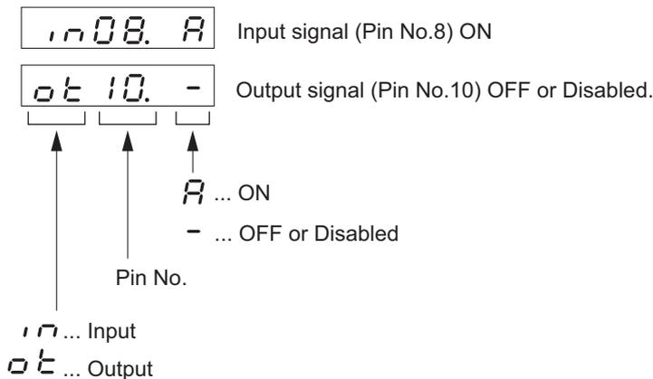
This indicates the status of the control input and output signals connected to CN1 pin.
