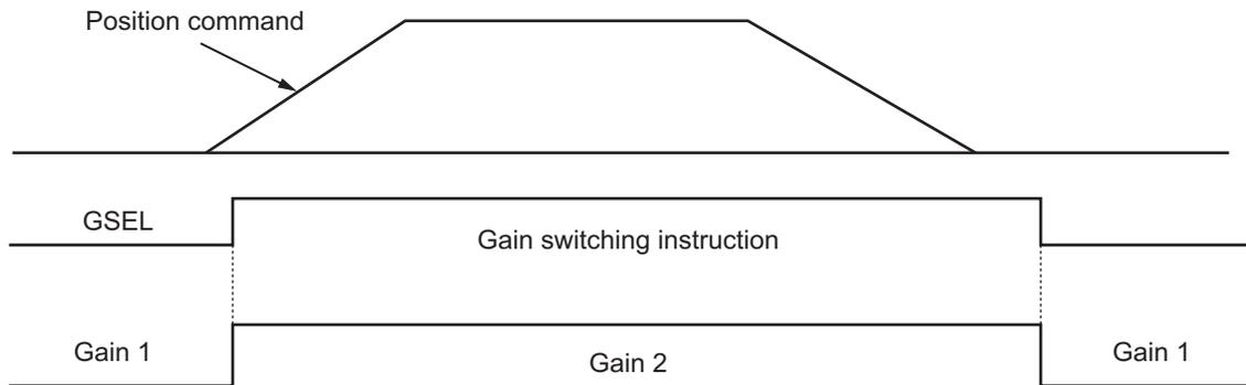
● **Gain Switching Mode = 3: Switching by Amount of Change in Torque Command**
