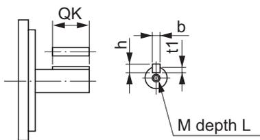
\*2 The tolerance is "h8" for R88G-HPG50□ or R88G-HPG65□.
