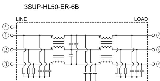
**Noise Filter for Brake Power Supply**
