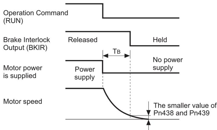
“TB” in the above figure is the setting time in Brake Timing During Operation (Pn438) (set value x 1 ms) or the time until the motor rotation speed falls to the setting speed or lower in Brake Release Speed Setting (Pn439), whichever is shorter.
