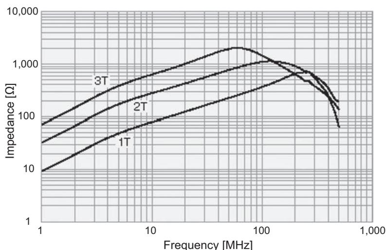
Refer to *External Dimensions* on page 4-30 and *Impedance Characteristics* on page 4-31 for information on the external dimensions and impedance characteristics of the ZCAT3035-1330 clamp core.
