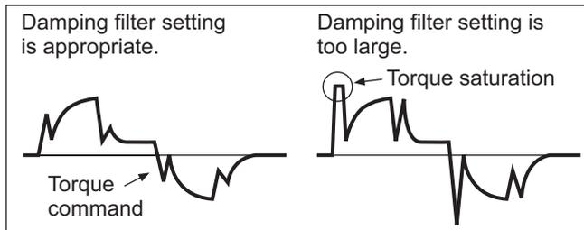
When Damping Frequency 1 (Pn214) is set, reduce this setting if torque saturation occurs or increase this setting to improve the operation speed. Normally 0 is set.
