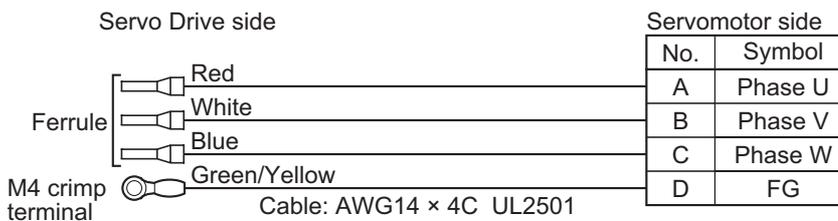
[Servomotor side connector]
