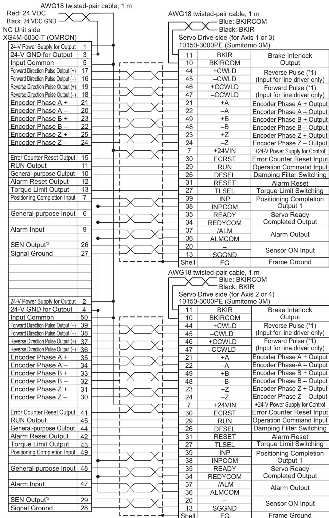
\*1 Connect the NC unit as shown here because it handles forward direction commands as CW-direction/phase-A advance pulses (which can be selected using the output pulse direction selection parameter).
