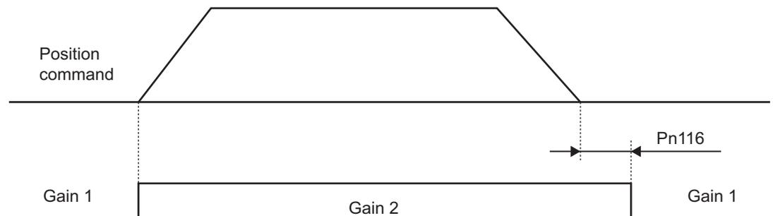
● **Gain Switching Mode = 8: Switching by Positioning Completion Signal OFF**
