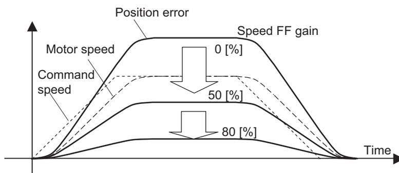
The position error in the constant speed range becomes smaller as the speed feed-forward gain increases.
