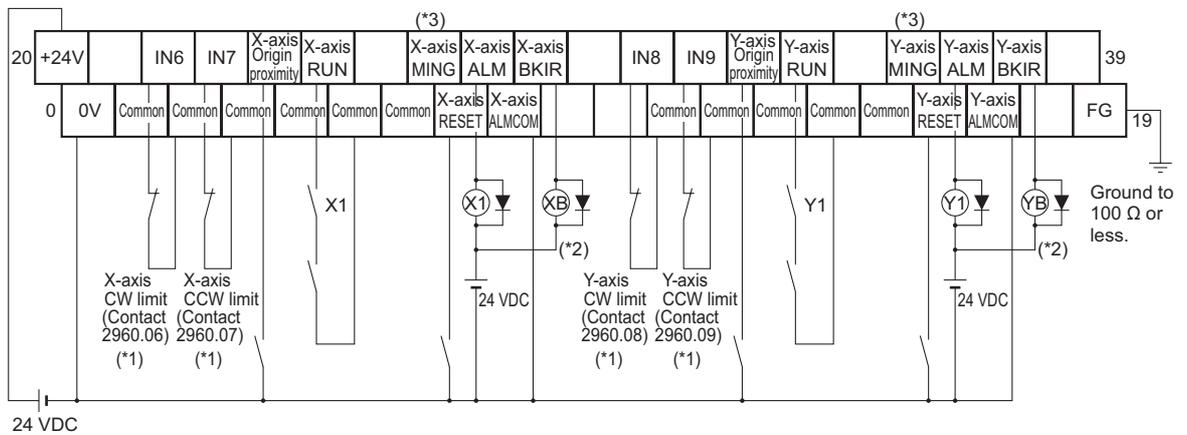
\*1 CW and CCW limit input signals can also be input to an input unit. For CJ2M, the CW and CCW limit input signals function with the following signals. CW: A540.08/CCW: A540.09 (Pulse output 0), CW: A541.08/CCW: A541.09 (Pulse output 1) Therefore, in ladder programming, use the actual input as CW and CCW limit input signals to output the following flag.
