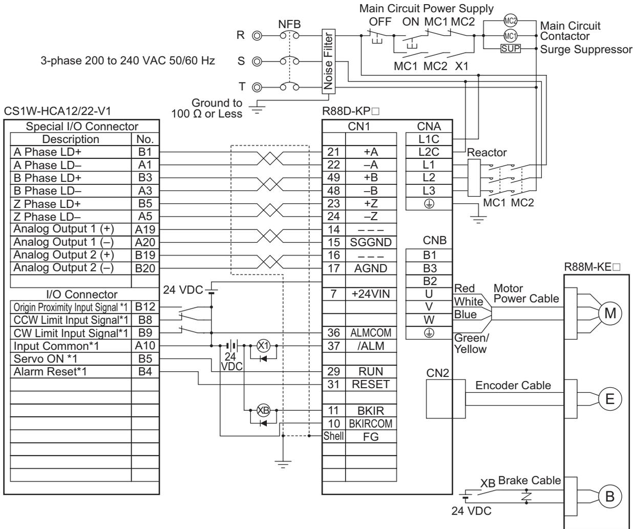
\*1 The I/O signals for the HCA12/22 vary depending on the allocations in the internal relay area. Change the wiring according to the allocations.
