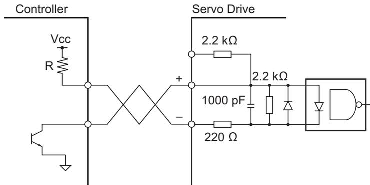
Select an appropriate Current Limit Resistor (R) for Vcc.
