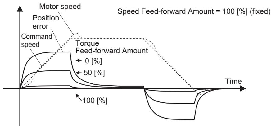
Torque feed-forward can reduce the position error in the range of constant acceleration/deceleration.
