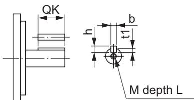
\*1 The tolerance is "h8" for R88G-HPG50□ or R88G-HPG65□.
