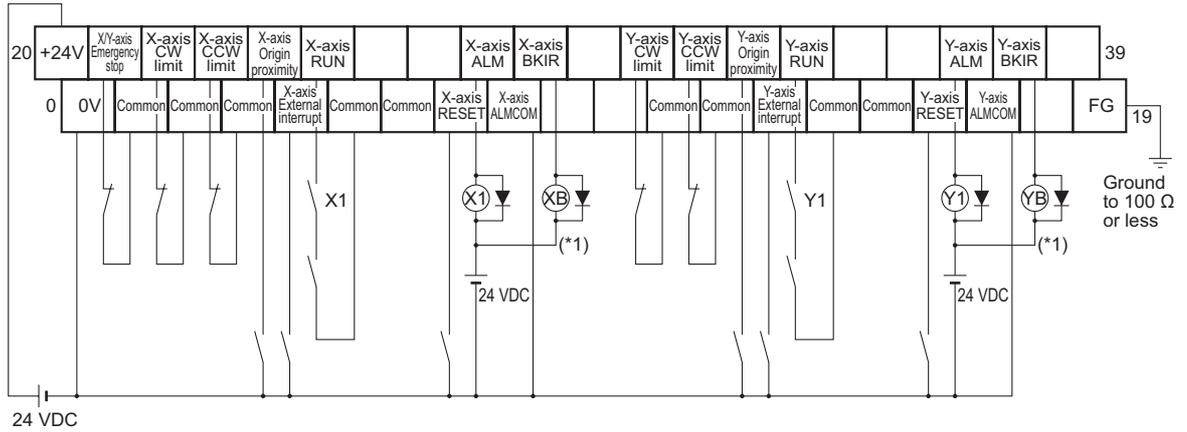
\*1 The XB and YB contacts are used to turn ON/OFF the electromagnetic brake.
