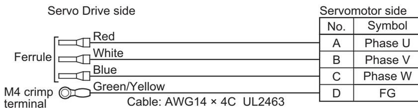
[Servomotor side connector]
