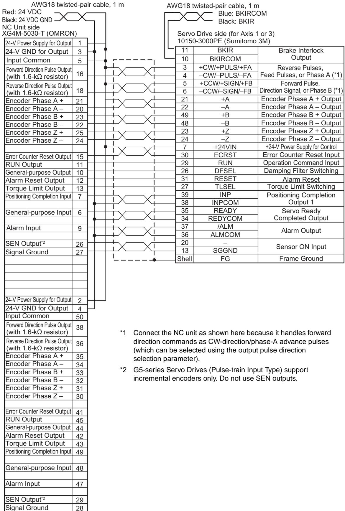
\*1 Connect the NC unit as shown here because it handles forward direction commands as CW-direction/phase-A advance pulses (which can be selected using the output pulse direction selection parameter).
