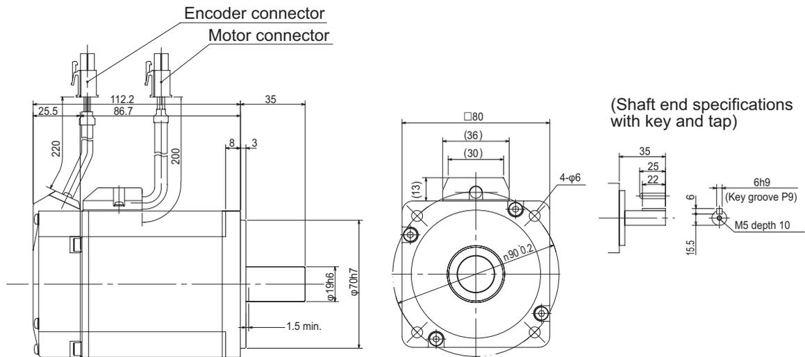
**Note** The standard models have a straight shaft. Models with a key and tap are indicated with S2 at the end of the model number.
