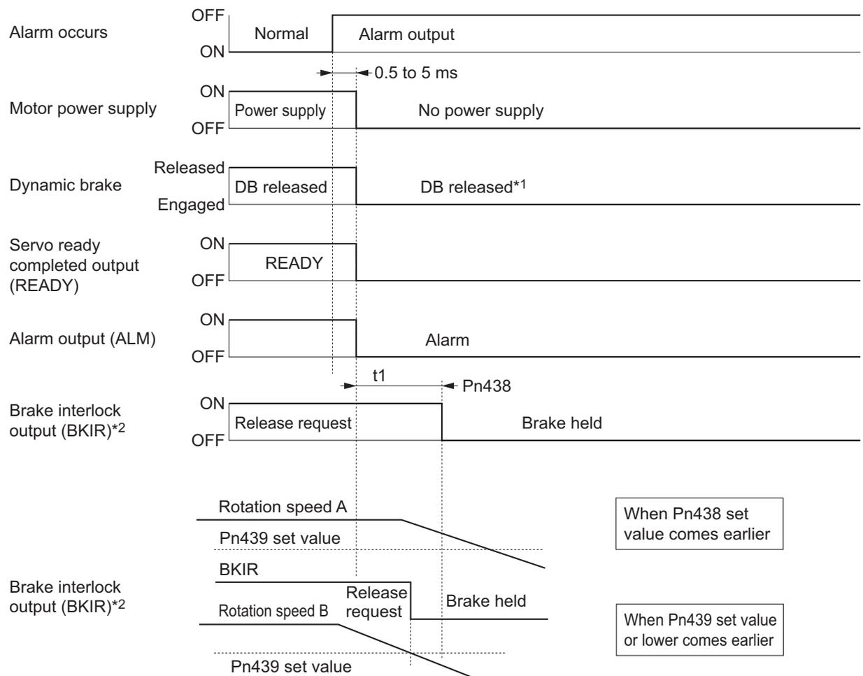
\*1 The operation of the dynamic brake when there is an alarm depends on the set value in Stop Selection with Servo OFF (Pn506).
