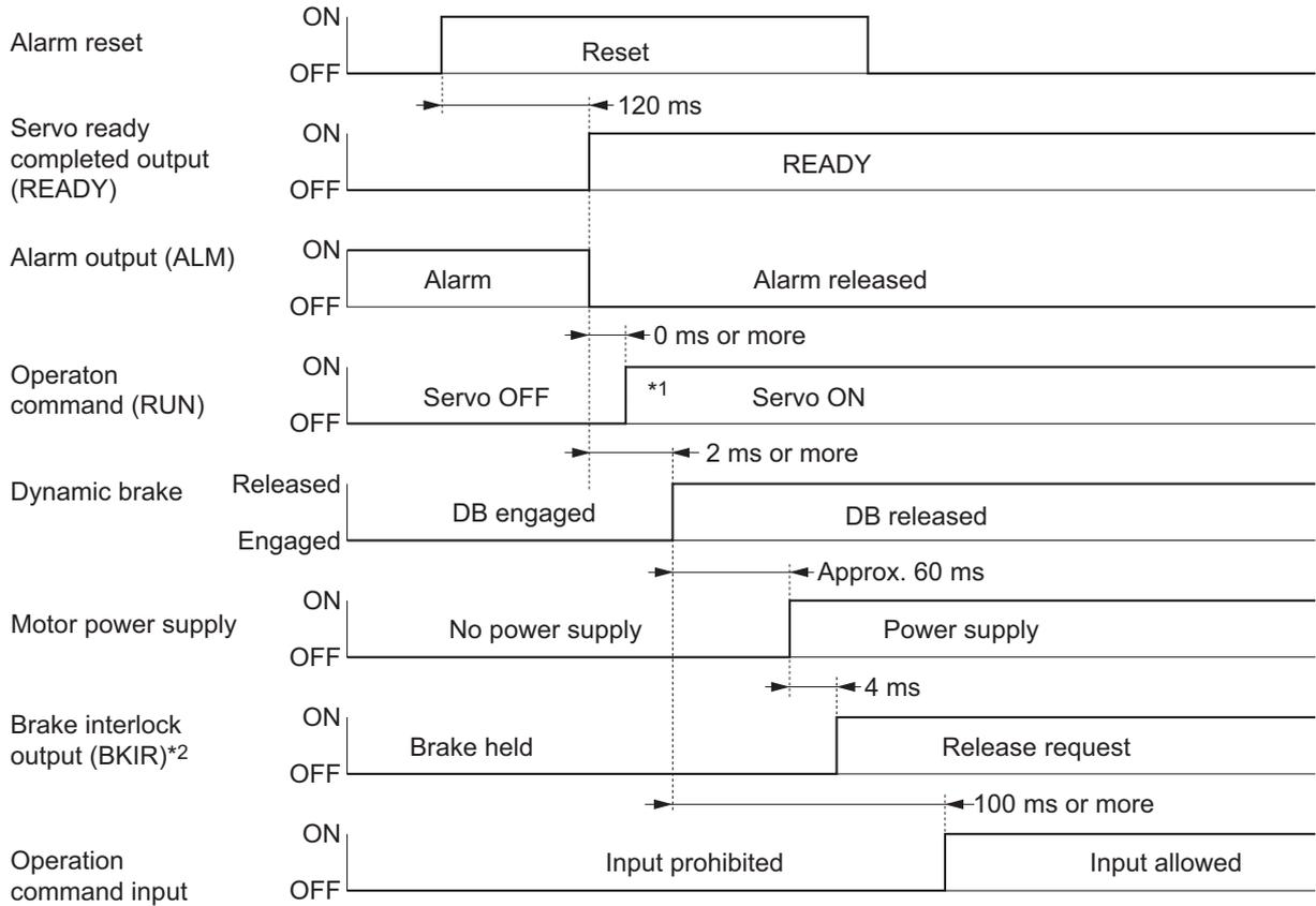
\*1 The servo does not turn ON until the motor rotation speed drops to approximately 30 r/min or lower.
