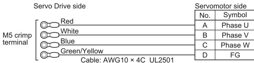
[Servomotor side connector]
