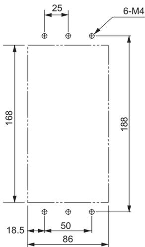
● Front Mounting (Using Front Mounting Brackets)
