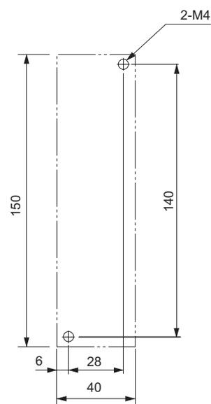
● Front Mounting (Using Front Mounting Brackets)
