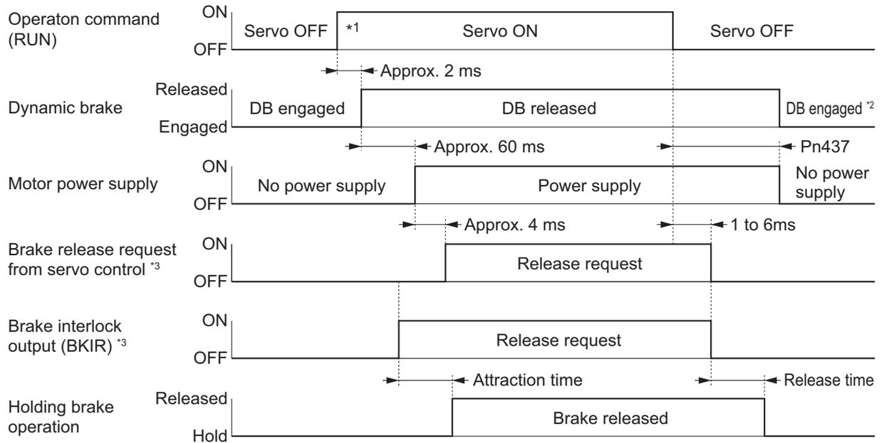
\*1 The servo does not turn ON until the motor rotation speed drops to approximately 30 r/min or lower.
