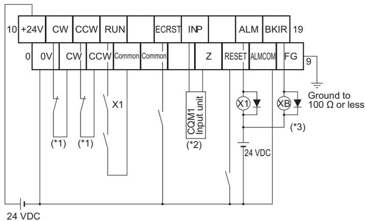
\*1 Use this signal to loop-back and input CQM1's output pulses into a high-speed counter.
