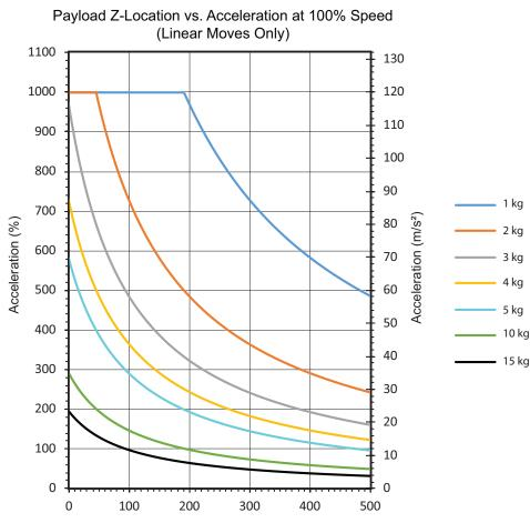
Payload Z-Location (mm) = Joint 3 Position + Payload Center of Gravity
