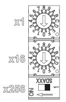
When the EtherCAT node ID is set with Sysmac Studio, it is retained in non-volatile memory and will persist after subsequent power cycles.
