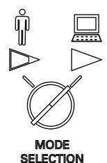
In Automatic mode, the robot can move unexpectedly. Ensure all personnel remain clear of the cell when Automatic mode is enabled.
