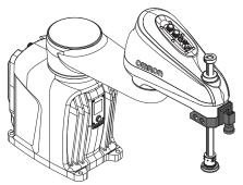
Use five M5 X 20 socket head cap screws with 2.5 N-m torque and Loctite 222 or equivalent thread locking compound when attaching the bracket to the robot.
