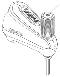
**11** Begin the lower bellows installation by sliding the bellows up the quill and then wrap it around the exterior of the robot housing.
