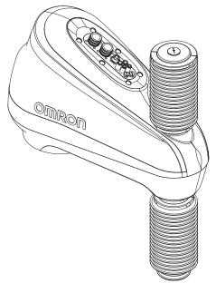
17 Place the large clamp on the tool flange bearing adapter. The bellows should be evenly positioned between the tool flange bearing adapter and the large clamp.
