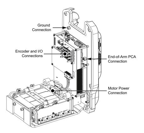
**5** After all internal connections have been removed, slide the amplifier chassis out of the robot base completely.
