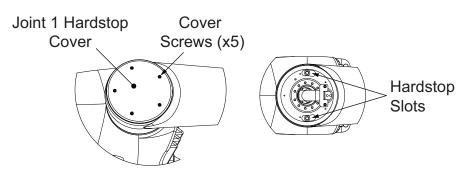
2 Move the inner arm to the desired position to expose the appropriate slot. Use the following figure to determine the Joint 1 position required to expose a specific hard stop slot. Positions in parenthesis represent the hardstop limit value.
