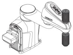
Bellows prevent debris or liquid from entering the internal compartment of the outer link, protect the Joint 3 quill, and prevent contamination of items external to the robot. This optional item is included for IP65 and Cleanroom rated robots.
