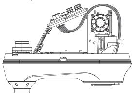
Place the pneumatic valve assembly at the mounting location shown below, and then insert two M4 x 30 screws with lock washers as shown in the following figure.
