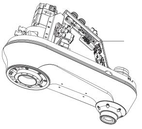
**10** Replace the plugs on the top of the Primary Interface Panel(ports 5 and 6) with two of the 6 mm fittings that were removed in the previous step.
