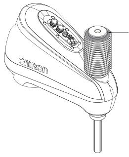
**8** Place the two halves of the large clamp on the upper bearing adapter. The bellows should be evenly positioned between the upper bearing adapter and the large clamp.
