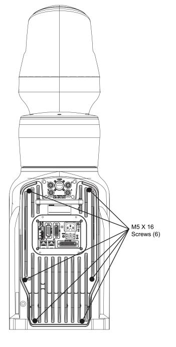
Carefully pull the amplifier chassis away from the robot base a small amount to expose internal harness connections. The assembly slides with guides in tracks.
