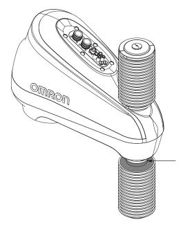
$\boldsymbol{12}$  Place the two halves of the small clamp around the robot housing.
