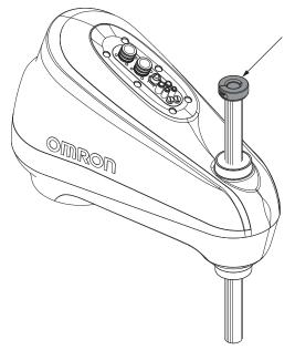
Slide the bellows down the quill and then wrap it around the exterior of the robot housing.Orientation of the bellows is not required because it is symmetrical.Take care to ensure the bellows is wrapped evenly and completely around the robot housing.
