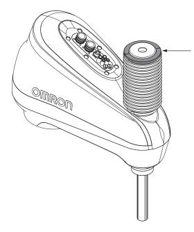
**2** Remove the bellows from the upper bearing adapter by pulling it down and off of the lip.
