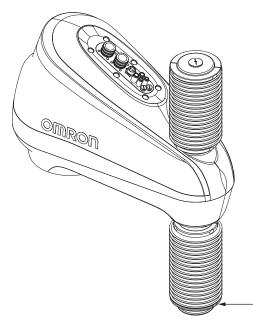
**18** Apply thread lock to the large clamp fasteners, insert, and tighten using a 2.5 mm hex key while ensuring that the bellows are completely seated and positioned between the large clamp and the tool flange bearing adapter. Tighten to a torque of 0.6 N-m. After the large clamp is secured, the bellows installation procedure is complete.
