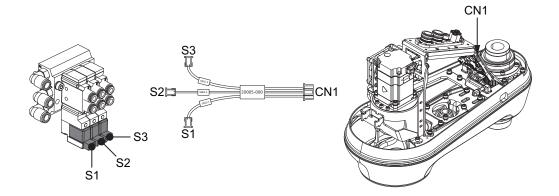
14 Secure the wire harness using supplied cable ties.Secure the wire harness to a rigid location that prevents it from interfering with moving parts such as a fan or belt.Trim any excess cable tie material using cutters.
