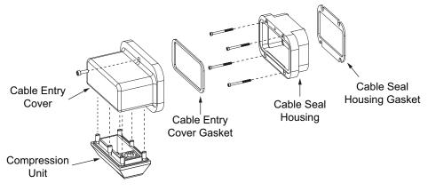
**1** Apply the provided Roxtec lubricant to the inside surfaces of the Compression Unit.
