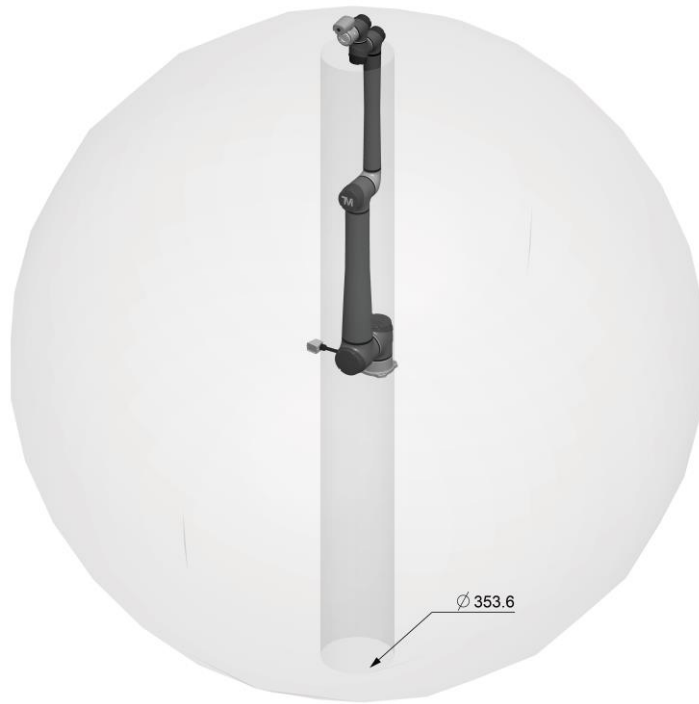
Figure 21: Pictorial view of TM6S Series Movement Range Diagram
