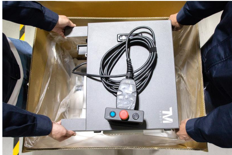
Figure 99: Moving the Control Box (2/2)
