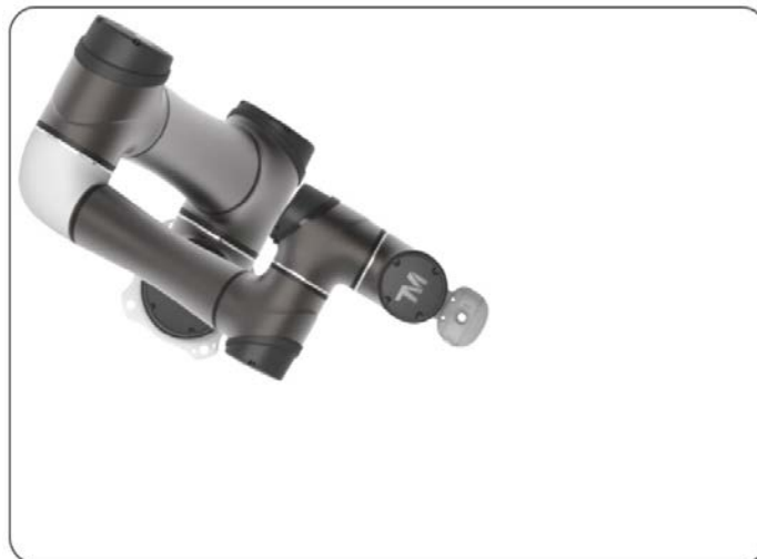
Figure 56: Top View of TM Robot Mounted on the AGV/AIV
