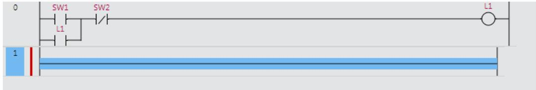
**3.** Insert the N.O. input *L1* as shown below.
