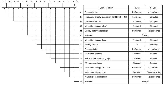
Bits 2 and 3 are not used when the PT is in NT20S or NT30/620 compatible mode.
