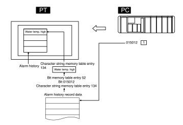
The PC bit allocated to the bit memory table entry for which the history property has been set is continually monitored: when the bit turns ON (1), the time, the number of times, and the contents of the character string memory table entry registered for the bit memory table entry are recorded in the alarm history record data.
