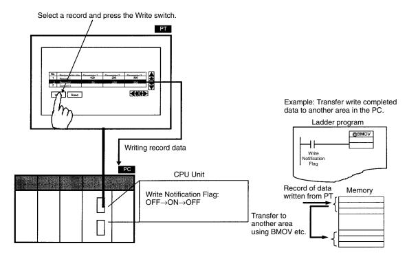
**Reference:** Recipe tables and recipe elements are stored in flash memory within the PT and memory (recipe data memory) that is backed up by a battery. (The Battery is an option for the NT21.) The way that the data is stored is explained below and illustrated in the diagram following.
