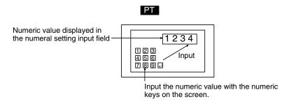
2. On confirming the input numeric value with the ENT key or doubt switch it is written to a numeral memory table entry.
