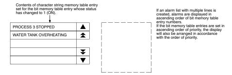
Since the message area is a touch switch, pressing the message causes the set image/library data to be displayed. At the same time, the pressed message is displayed in the ON color.
