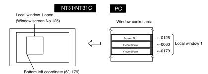
Opening/Closing and moving a window by the operation of window control area
