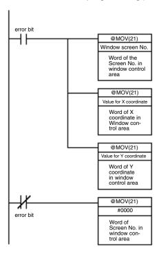
With this ladder program, the specified window is displayed at the designated position when the error bit comes ON, and the window is closed when the error bit goes OFF.
