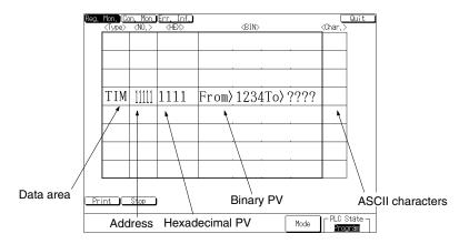
With the NT631/NT631C, the PVs of up to 8 words can be displayed simultaneously.
