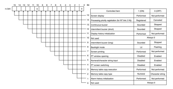
The backlight mode bit (bit 8) is not supported by the NT631. The screen printing bit (bit 7) is not supported by the NT21.
