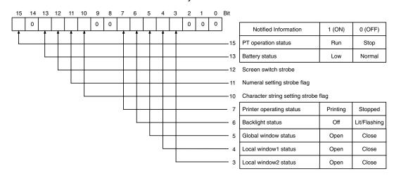
The printer operating status (bit 7) is not supported by the NT21.
