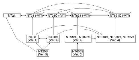
\* The following downward screen data conversions are not possible: V2 or V3 models → V1 models or models without a -V□ suffix; or V1 models → models without a -V□ suffix. The following upward screen data conversions are possible: Models without a -V□ suffix → V1, V2 or V3 models; or V1 models → V2 or V3 models.
