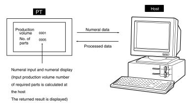
When the numeral was input on PT, numeral input notify command (sent from PT to host) is issued from the PT. At the host, numeral data was taken out and processed, then it is written to the PT by the numeral memory table write command (sent from host to PT).
