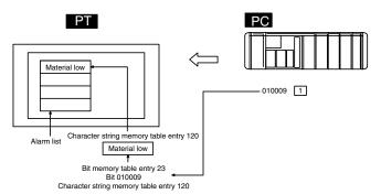
When the PC bit comes ON (1), the contents of the character string memory table entries registered for the bit memory table entries are displayed in the alarm list. When the bit returns to the OFF (0) status, the character string memory table display is automatically cleared.
