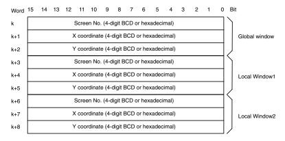
With the program in the host, read out window screen number, X coordinate and Y coordinate in a window control area that corresponds to the window of which display status is to be checked.
