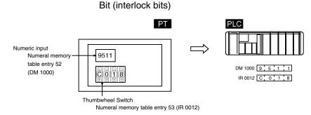
Allocate any desired words in the PC to the numeral memory table entries. When a value is input or changed with the numeric input or thumbwheel switch, the new value will be written to the numeral memory table entry and the contents of the words allocated in the PC will be changed automatically. This function allows word PVs to be changed easily from the PT.
