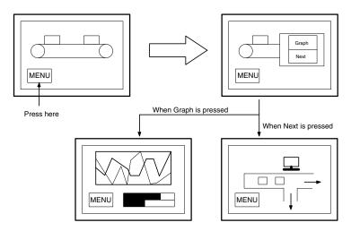
• The window can also be used as a sub screen for displaying a detailed information as required.
