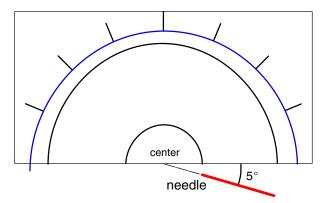
Display Method of the Area Between the Present Value and the 0% Value Present value of an analog meter is displayed using needle or fill as a display type. If you specify needle, the present value is showed as a needle, if you specify fill, the area between 0% and the present value will be tiled in selected foreground color.
