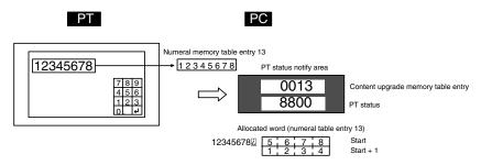
Reference: When the PT is set to NT20S or NT30/620 compatible mode, the word configuration is identical to that of the earlier NT20S, NT30, NT30C, NT620S, NT620C, and NT625C PTs.
