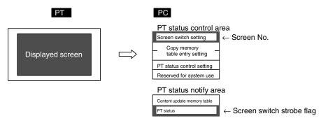
Reference: When NT20S or NT30/620 compatible mode is being used, the current screen number occupies the first word of the PT status notify area and the word containing the PT status notify bits is shifted down one word. (Refer to page 451.)
