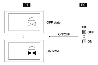
1, 2, 3... 1. Create figures depicting the valve when open (A in the figure below) and the valve when closed (B in the figure below), either by using library data (fixed display graphic) or image data (comprised of dots).
