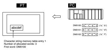
Allocate any desired words in the PC to character string memory table entries. If the contents of the allocated words are changed while the character string memory table data is being displayed on the screen as text, the corresponding display on the screen will also change automatically. This function allows any desired message to be displayed easily.
