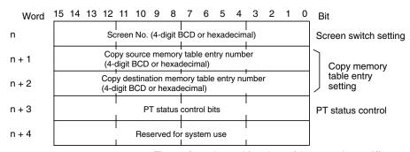
The configuration and functions of these words are different when the PT is in NT20S or NT30/620 compatible mode.
