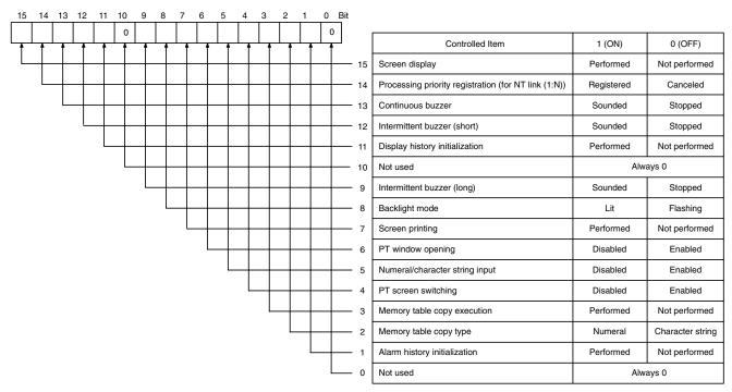
Bits 2 and 3 are not used when the PT is in NT20S or NT30/620 compatible mode. Bit 7 is not supported by the NT21.
