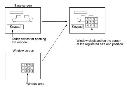
Windows can be called anytime, regardless of which screen is currently displayed. It is possible to display multiple windows (max.: 3) on the same screen, and to open, close or move windows by the control from the host.
