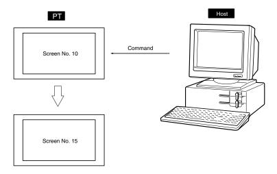
Use PT memory write command (sent from host to PT) for this case since it is necessary to write new screen number to the first word in PT control area.
