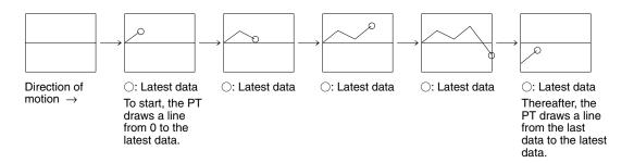
The drawing results with each Direction setting are indicated below.
