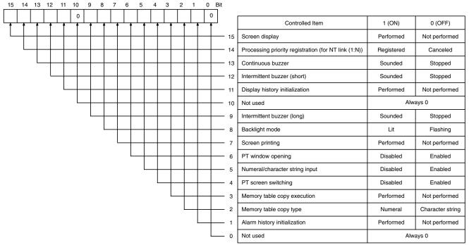
Bits 2 and 3 are not used when the PT is in NT20S or NT30/620 compatible mode. Bit 7 is not supported by the NT21.
