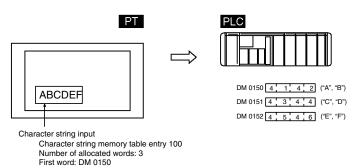
Allocate any desired words in the PC to character string table entries. When text is input with a character string input, the new character string will be written to the character string memory table entry and the contents of the words allocated in the PC will be changed automatically. This function allows text to be written from the PT to the PC easily.
