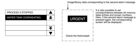
4. When a message displayed in reverse video is pressed again, the display will switch to the screen with the set screen number.
