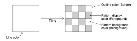
Reference: When a lamp, a touch switch, and a graphic are displayed in color, part of the frames of the display elements may be invisible because of the combination of the background, outline, and tiling colors. This is a phenomenon peculiar to a color LCD, not a failure of the system. In such a case, change the color combination.
