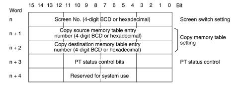
**Reference:** The configuration and functions of the PT status control area are different when the PT is set to NT20S or NT30/620 compatible mode. Refer to Appendix C for details on the NT20S and NT30/620 compatible modes.
