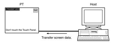
**Reference:** Do not touch the touch panel while screen data is being transferred by the memory link online transfer function. (Do not press the Exit touch switch either.)
