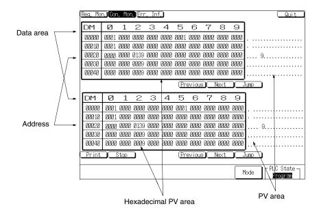
With the NT631/NT631C, two tables of 50 words (10 words  $\times$  5 rows) can be displayed simultaneously for a total of 100 words.
