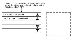
If an alarm list with multiple lines is created, alarms are displayed in ascending order of bit memory table entry numbers. If the bit memory table entries are set in ascending order of priority, the display with the order of priority.
