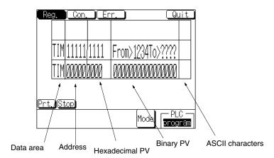
With the NT31/NT31C, the PVs of up to 3 words can be displayed simultaneously.
