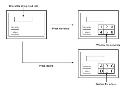
Reference: In order to make numeral/character string settings, a key to confirm the input numeric value or character string is required. Assign the ENT input key-control or Enter ( ) key to a touch switch to create this key.
