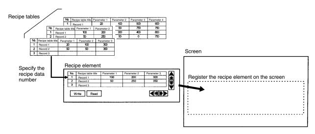
Sending Recipe Tables and Recipe Elements Using the Support Tool Send recipe tables (i.e., entire sets of recipe data) and recipe elements created as shown above from the Support Tool to the PT in application units (i.e., send all screen data in a single operation).
