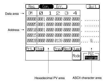
With the NT31/NT31C, the PVs of up to 25 words (5 words  $\times$  5 rows) can be displayed simultaneously.
