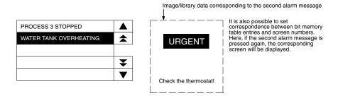
5. When the reverse video message is pressed, the screen changes to the screen with the set screen number.
