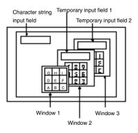
In the example above, window 2 is a focus window. All the input indicated below is performed to a temporary input field on window 2.
