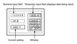
However, if there is not even one numeral setting input field (numeric key type) or character string input field on the base screen, the temporary input field will not be displayed (cannot be used).
