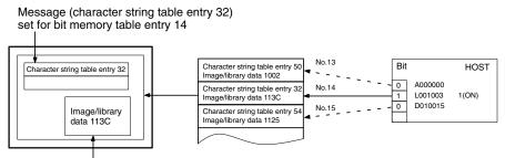
When the message displayed is pressed, the image/library data (113C) set for bit memory table entry 14 is displayed.
