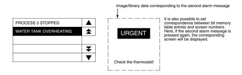
4. When a message displayed in reverse video is pressed again, the display will switch to the screen with the set screen number.
