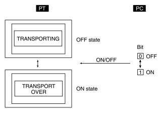
Register a normal lamp for the screen with the following settings.
