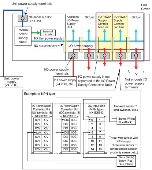
\*1. Wire colors have been changed according to revisions in the JIS standards for photoelictric and proximity sensors. The colors in parentheses are the wire colors prior to the revisions.
