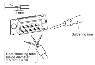
**4** Return the heat-shrinking tube to the soldered portion, then heat the tube to shrink it with a heat gun.
