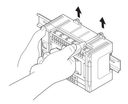
2 Remove the CPU Unit from the DIN Track. Pull the Unit straight forward to remove. Be careful not to drop it.
