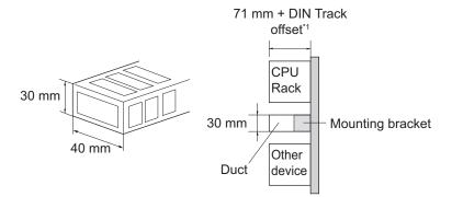
\*1. It varies depending on the DIN Track to be used. Refer to *Installation Dimensions* on page 5-34 under 5-3-13 Assembled Appearance and Dimensions on page 5-34 for details. It corresponds to the dimension (B).
