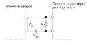
V<sub>CC</sub>: Power supply voltage V<sub>ON</sub>: ON voltage of DC input V<sub>OFF</sub>: OFF voltage of DC input I<sub>ON</sub>: ON current of DC input I<sub>OFF</sub>: OFF current of DC input R<sub>IN</sub>: Input resistor of DC input
