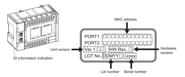
Note The hardware revision is not displayed for the Unit that the hardware revision is in blank.
