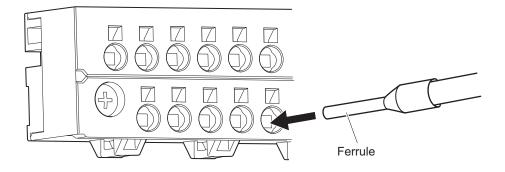
After you make a connection, make sure that the ferrule is securely connected to the terminal block.
