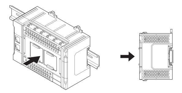
4 Press the DIN Track mounting hooks down to the locked position. After mounting, make sure that the CPU Unit and the End Cover are securely mounted on the DIN Track.
