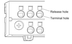
The above figure shows the output terminal block at the bottom. For the input terminal block, turn it upside down.
