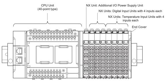
The widths of the Units in the example CPU Rack configuration and the total configuration width are given below.
