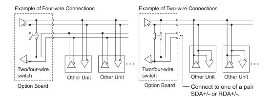
Set a terminating resistance if it is the end of transmission circuit.
