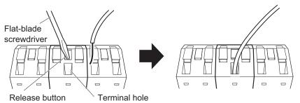
To remove the wire, press in the release button with a thin flat-blade screwdriver, and pull out the wire while it is unlocked.
