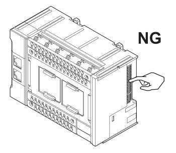
Do not write anything with ink within the restricted region of the CPU Unit that is shown in the following figure. Also do not get this area dirty. When the Unit is installed or removed, ink or dirt may adhere to the pins in the NX bus connector, which may result in malfunctions in the Unit.
