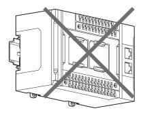
Mounting with the DIN Track Installed Vertically
