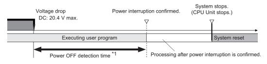
\*1. The power OFF detection time is 2 to 8 ms.
