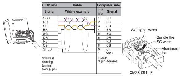
Example: When using cables and devices that you used with CS/CJ/CP Series.
