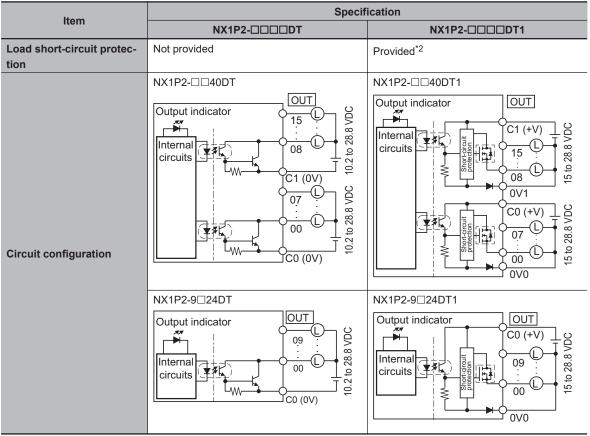
\*1. The internally consumed current from I/O power supply. The current flows from the common terminal Cn (+V) to the 0Vn terminal. The current consumption of any external load is excluded.
