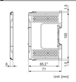
\*1. The dimension from the attachment surface of the DIN Track to the front surface of the end cover.
