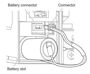
**4** Press in the battery harness and attach the battery cover.
