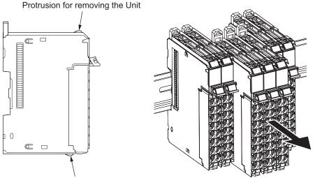
Protrusion for removing the Unit
