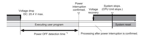
\*1. The power OFF detection time is 2 to 8 ms.
