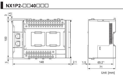
\*1. The dimension from the attachment surface of the DIN Track to the front surface of the CPU Unit.
