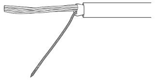
Remove the insulation from each core wire using a stripper.Cover the braided shield with a heat-shrinking tube (3.0 dia.), and heat the tube to shrink it in place.
