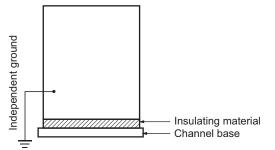
Example: Insulating and Grounding an Enclosure
