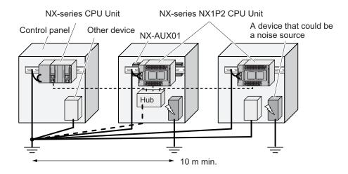
b. Connecting devices and noise sources to a common earth electrode
