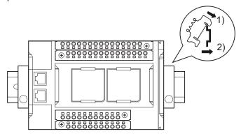
To remove an End Plate 1) insert the tip of a flat-blade screwdriver into groove "a" and 2) use "b" as a fulcrum and lift the end of the screwdriver, as shown in the following diagram.
