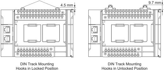
If the DIN Track mounting hooks are pulled up, they are in the unlocked position. If the DIN Track mounting hooks are pressed down, they are in the locked position. Use a flat-blade screwdriver to pull up the DIN Track mounting hook on the Unit to release the locked position.
