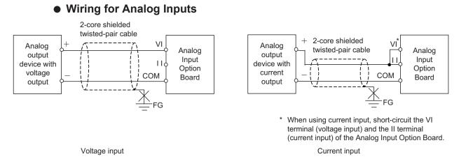
However, if noise affects the Unit, ground the end of the shield on the Input Unit side. You can use the NX-TBX01 Shield Connection Unit to ground more than one shield.
