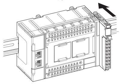
**3** Press the NX Unit with a certain amount of force against the DIN Track until you hear the DIN Track mounting hook lock into place.
