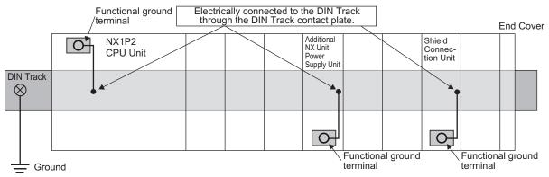
If the surface of the DIN Track is treated to produce an insulating material (e.g., anodized aluminum), the DIN Track contact plate will not be electrically connected to the DIN Track even if they are in physical contact.
