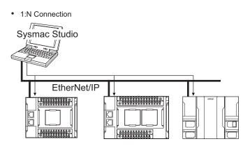
· Directly specify the IP address of the remote device.
