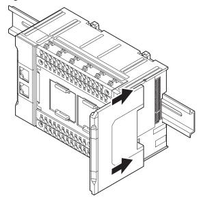
**2** Press the End Cover firmly against the DIN Track until you hear it lock into place on the DIN Track.
