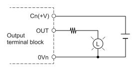
In countermeasure 1, the current consumption from I/O power supply is increased although the voltage supplied to the load L is not decreased.
