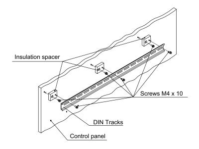
DIN Track Insulation Spacers NX-AUX01 (OMRON Corporation) Three Spacers are included in one model.
