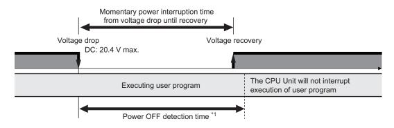
\*1. The power OFF detection time is 2 to 8 ms.
