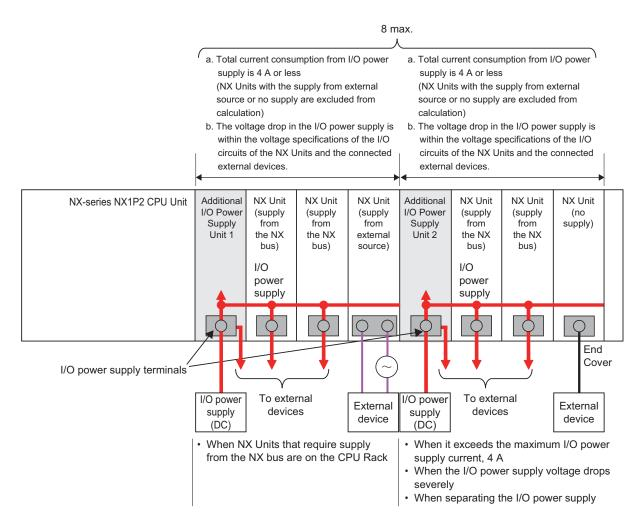
I/O power supply current consumption of each Unit
