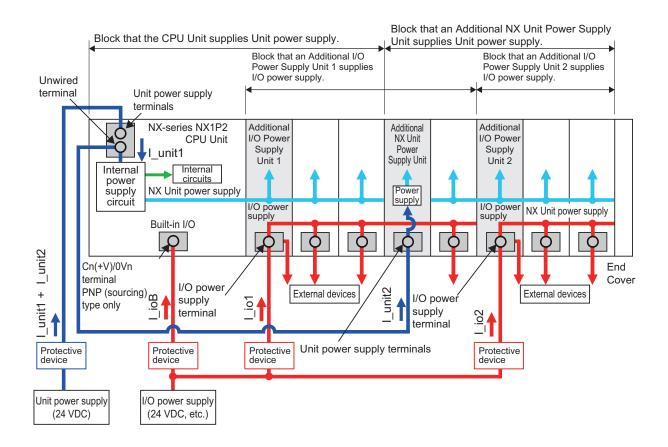
When Total Current Consumption for All Blocks Does Not Exceed the Rated Current In this example, the current consumption from each power supply is as follows: Current consumption from Unit power supply: 1 unit1 + 1 unit2 ≤ Lowest rated current
