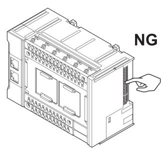
Do not write anything with ink within the restricted region of the CPU Unit that is shown in the following figure. Also do not get this area dirty. When the Unit is installed or removed, ink or dirt may adhere to the pins in the NX bus connector, which may result in malfunctions in the Unit. Refer to the user's manual for the connected NX Unit for information on the restricted region for the NX Unit.
