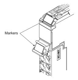
The marker attachment locations on the NX Units depend on the type of external connection terminals. Refer to the user's manual for the NX Units that you will use for the marker attachment locations.
