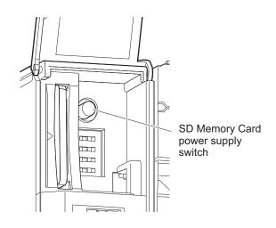
**2** Press the SD Memory Card after you confirm that the SD BUSY indicator (lit while SD Memory Card access is in progress) and SD PWR indicator (lit while SD Memory Card power is supplied) are no longer lit.
