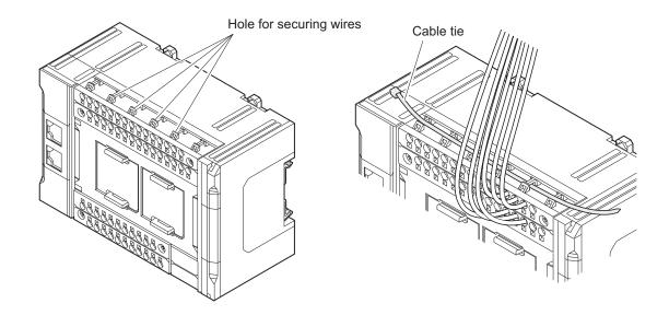
**3** Bundle five to six wires with a cable tie and secure them to the screwless clamping terminal block.
