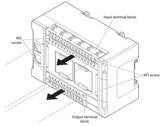
These screws are the self-raising screws, so the terminal block is raised when they are loosened. Loosen the right and left screws alternately if they are hard to loosen.
