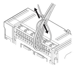
Secure wires within the range of 30 mm from the screwless clamping terminal block. Also, leave spaces above and below the CPU Rack to ensure ventilation, as shown in the following figure.
