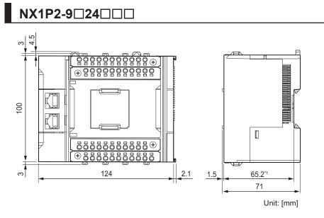
\*1. The dimension from the attachment surface of the DIN Track to the front surface of the CPU Unit.
