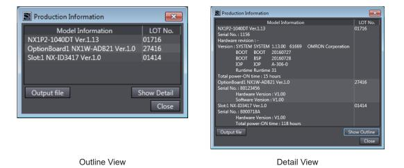
The information that is displayed is different for the Outline View and Detail View. The Detail View displays the unit version, hardware version, and software versions. The Outline View displays only the unit version.
