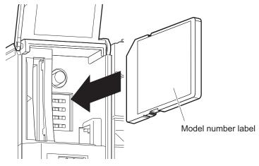
**3** Push the SD Memory Card securely into the compartment.
