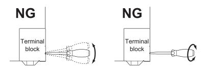
The angle at which you insert a screwdriver in the release holes on the screwless clamping terminal blocks of the CPU Unit is different from that on the screwless clamping terminal blocks of NX Units. Check the wiring method for the NX Unit and perform wiring correctly. Refer to the user's manual of the specific NX Unit for how to wire an NX Unit.
