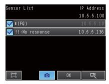
3 Select the sensor that you want to connect and touch [OK]. (The sensor is reconnected.)
