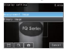
You can select from Measurement image and Binary image. (Default : Measurement image)
