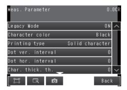
The [Legacy Mode] allows for Scene data, or Dictionary data created with software versions older than ver. 2.10 to be usable with ver. 2.02, or later software. The Dictionary data created with the old software version can only be used with Scene data also created from the old software version.
