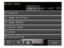
2 Press the parameter for which to log data to select it.
