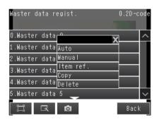
[Auto]: Registers a character string from an actual 2D code in the master data. The procedure is essentially the same as the procedure for teaching in step 2.
