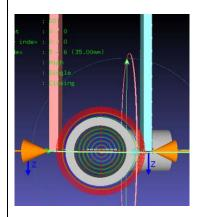
If the position of the hand causes a collision with the workpiece as shown in the figure on the right, the fingers will be shown in yellow. In this case, adjust the position to prevent collisions.
