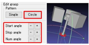
In some condition, the robot may not reach the set grasp point. Add grasp points considering the workpiece's orientation and the robot's rotational range limit.
