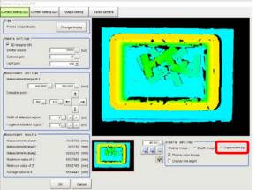
If you see only a black image in the window, check the box for "Captured Image" in the "Display setting" at the bottom right of the screen and confirm whether you can observe the projected mesh pattern image on the target object.
