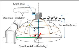
Set distance from 3D vision camera to the handeye calibration target in "Ref radius"
