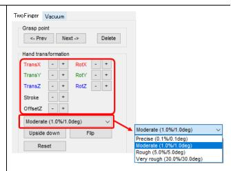
Use the guide on display to adjust the position so that the left and right fingers are equidistant from the workpiece.
