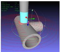
The Grasp point location and posture is adjusted by using "Hand transformation" buttons. The function of the button are as follows.
