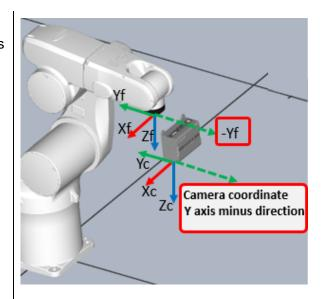
4 Open "Target settings" tab to set the calibration target pose and posture which are search result of the "3D Search" unit result.
