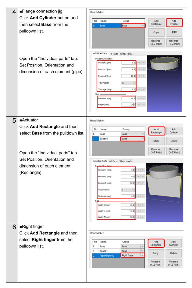
Open the "Individual parts" tab. Set Position, Orientation and dimension of each element (Rectangle)
