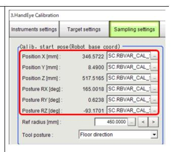
During the Hand-eye calibration procedure the robot moves half sphere trajectory from "Calib. Start pose" with keeping the calibration target in center of the 3D camera view.
