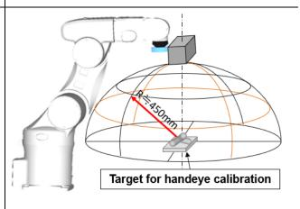
Adjust the position of the robot so that the hand-eye calibration target to capture is near the center of the field of view.
