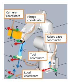
For each coordinate system, the orientation of each axis differs depending on the robot manufacturer and axis configuration. For the detailed definition of the coordinate systems, please refer to the manual for your robot.
