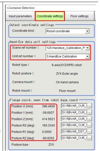
Confirm that "Flange coord. seen from robot base coord" values are same as the robot current position.
