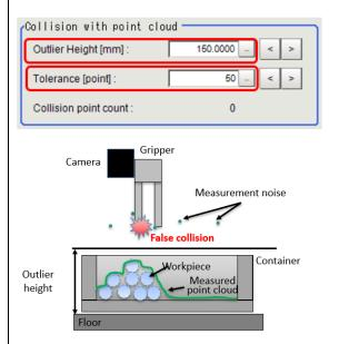
Set "Tolerance" for ignoring point cloud collision with hand caused by measurement noise.
