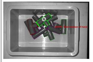
If the number of grasp candidates is 0 even though a workpiece is detected in 3D Search, check the following to narrow down the causes.
