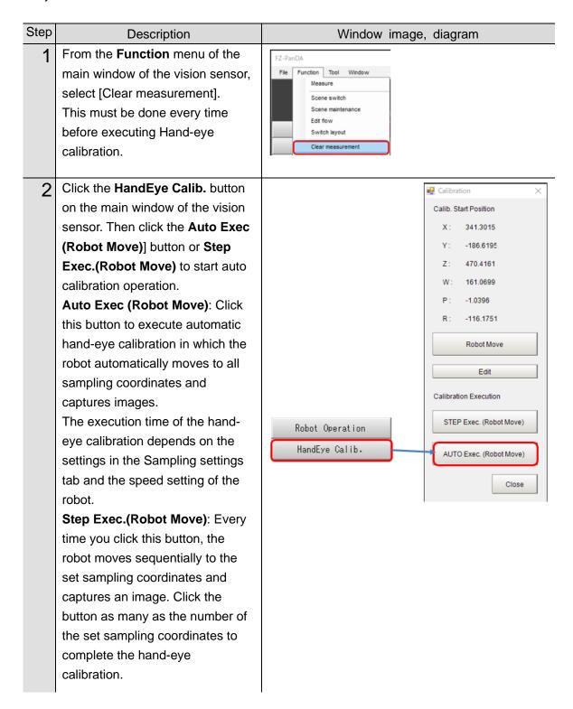
The progress of the hand-eye calibration is indicated as *Number* of executed steps/Total number of steps in **Step** in the detailed result display window.
