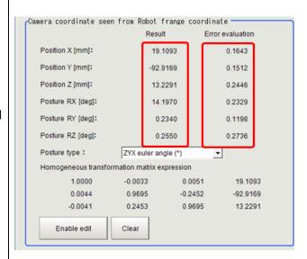
The origin of the actual camera coordinate system is located inside at about a few more than 10 mm from the surface of the 3D vision camera. Therefore, the indicated result for Position Z will be 10 and a few mm smaller than the setting.
