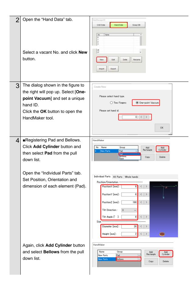
Open the "Individual parts" tab. Set Position, Orientation and dimension of each element (Bellows).
